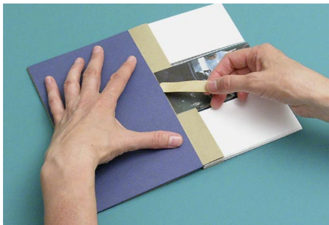
Figure 33, Removing release paper from double stick after insertion of spine into cover.
