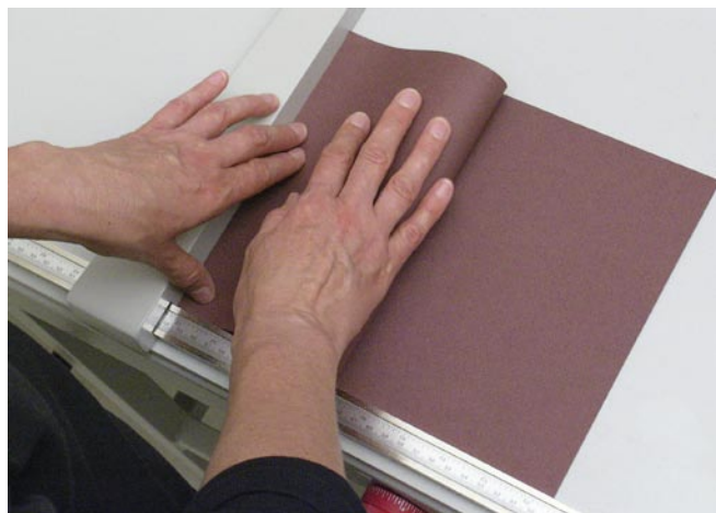
Figure 42, Using the bed of a Kuttrimmer as guide for precise folding.
